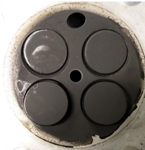
Figure 5.12: Cylinder head painted with black color.
